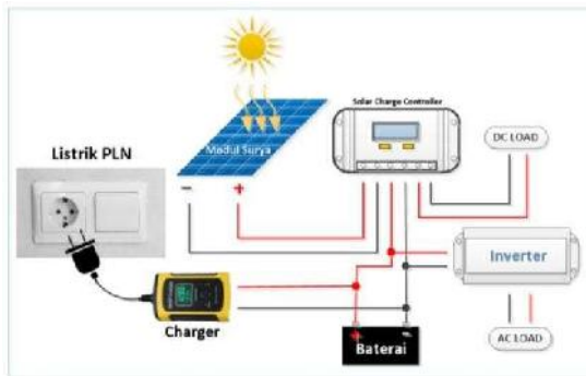
Gambar 8. Skema sistem power station mobile
