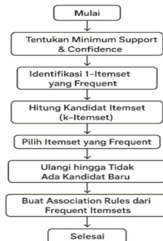
**Gambar 3.** Diagram Alur Algoritma Apriori
