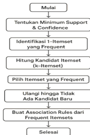
Gambar 3. Diagram Alur Algoritma Apriori
