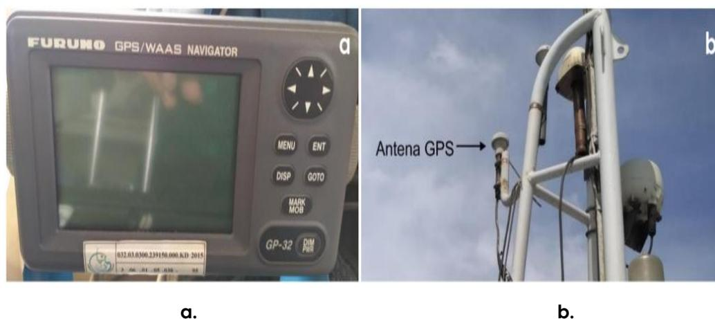
**Gambar 3.** (a) *Display Unit*; (b) *Antena GPS*
