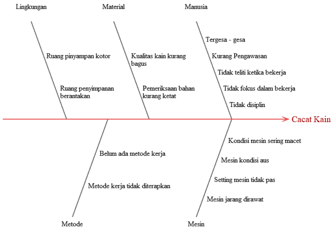
Gambar 5. Fishbone Diagram Cacat Kain
