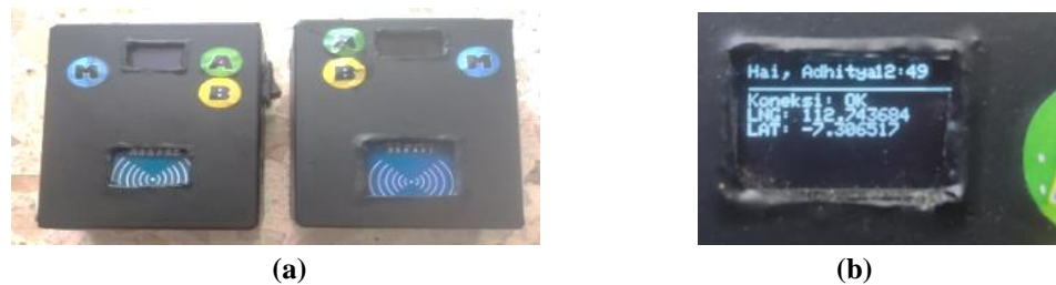
Figure 2. (a) Tracker Tool Prototype; (b) GPS tracking status information display
