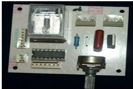
Figure 7. Dimmer set module [15]
