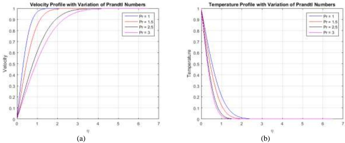
**Figure 3. (a) Velocity Profile and (b) Temperature Profile with Variation of Prandtl Numbers**
