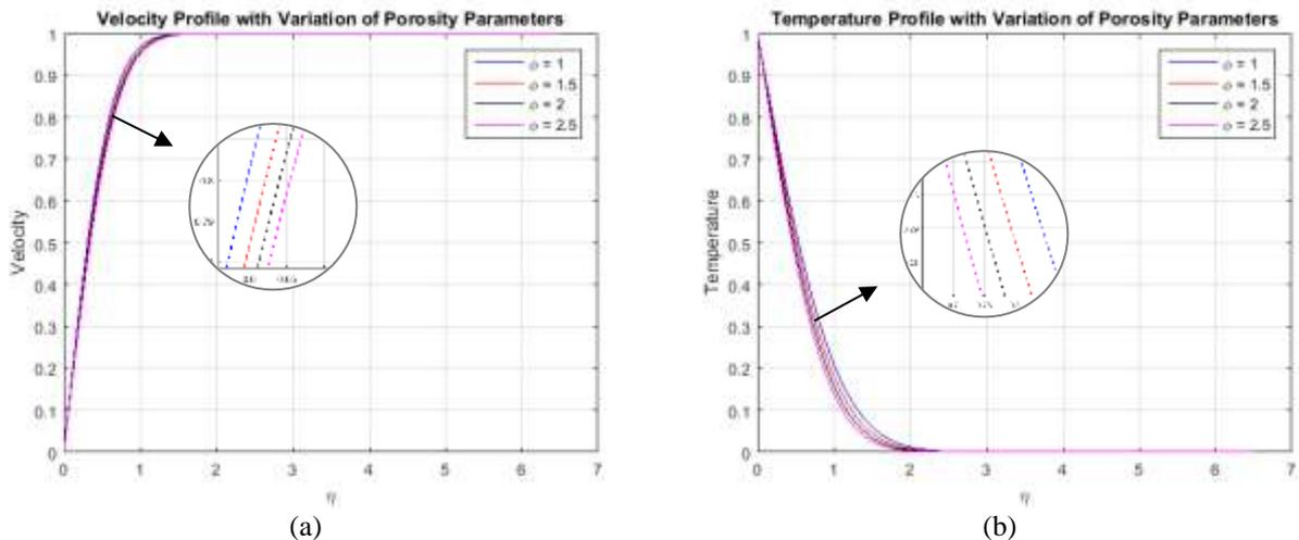
**Figure 4. (a) Velocity Profile and (b) Temperature Profile with Variation of Porosity Parameters**
