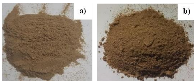
Figure 1. Water hyacinth powder: a) before, and b) after activation
