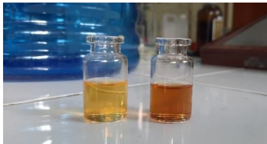
Figure 6. Color of Bio-oil Before Upgrade (Right) and After Upgrade (Left)
