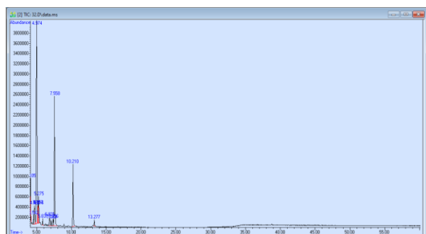
Figure 3. Liquid Smoke GC Chromatogram Pyrolysis results (after rotary evaporator)
