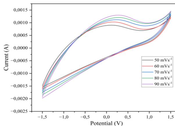
Figure 4. Voltammogram of determining optimum scan rate
