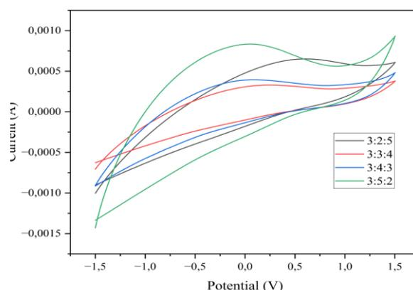
Figure 2. Voltammogram of determining optimum electrode composition
