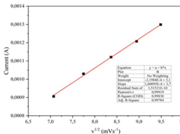
Figure 5. Linear curve between the square root of scan rate and  $I_p$
