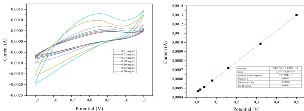
Figure 6. (a) Voltammogram of different concentrations (b) Calibration curve
