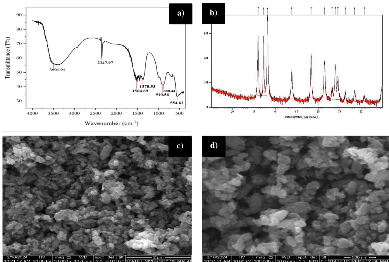
Figure 1. Characterization of ZnO nanoparticles (a) FTIR Spectrum of ZnO nanoparticles (b) Diffraction pattern of ZnO nanoparticles (c) SEM image of ZnO nanoparticles (50.000x magnifications) (d) SEM image of ZnO nanoparticles (100.000x magnification)
