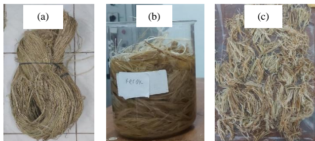
Figure 1. (a) SRK raw materials that have not been pretreated, (b) alkalization process using 5% NaOH solution for two hours at room temperature, and (c) the resulting SRK after being dried at room temperature for two to three days and cut into pieces
