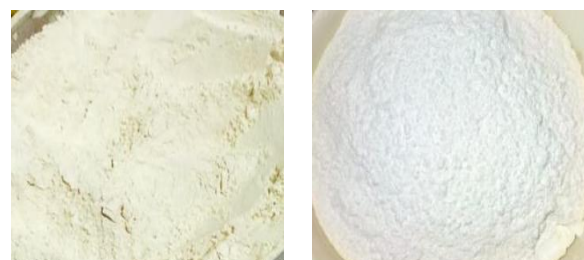
Figure 2. Chicken Egg Shell Calcination (a) \text{CaCO}_3 ; (b) \text{CaO}
