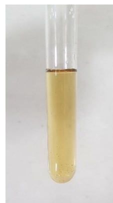
Figure 1. Visual appearance of silver nanoparticles (AgNp) colloidal synthesized by the \text{NaBH}_4 reduction method.
