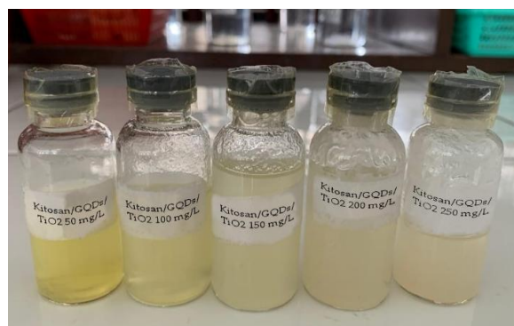
Figure 1. Visual appearance of CS/GQDs/TiO 2 composite solutions with different TiO 2 concentrations before film formation
