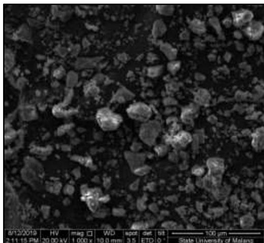
Figure 5. SEM of  $\text{Fe}_3\text{O}_4$  encapsulated PEG 4000
