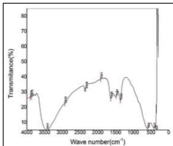
Figure 2. FTIR Spectra of Fe<sub>3</sub>O<sub>4</sub> nanoparticles
