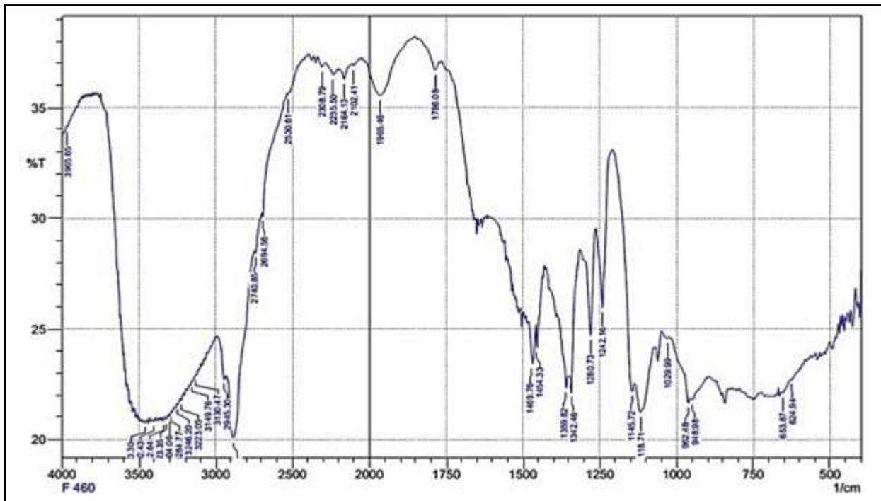
Figure 3. FTIR Spectra of Fe<sub>3</sub>O<sub>4</sub> nanoparticles encapsulated PEG 4000
