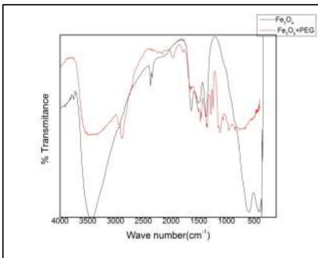
Figure 4. FTIR combination of Fe<sub>3</sub>O<sub>4</sub> and Fe<sub>3</sub>O<sub>4</sub> nanoparticles encapsulated PEG 4000
