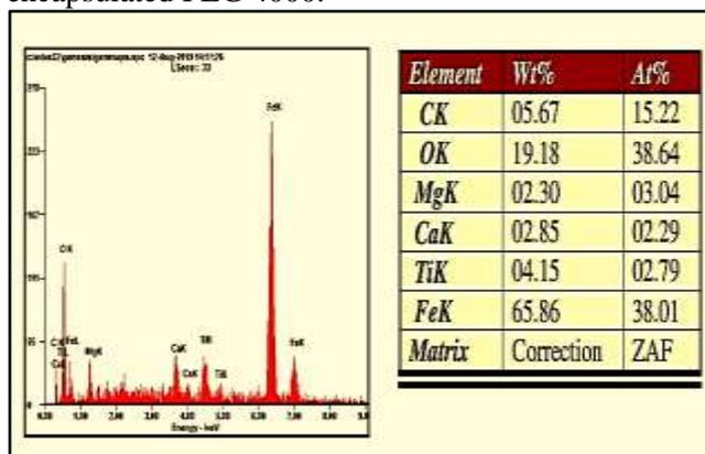
Figure 6. EDS of  $\text{Fe}_3\text{O}_4$  encapsulated PEG 4000
