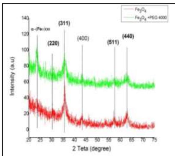
Figure 1. Diffraction peaks of the nanoparticle Fe<sub>3</sub>O<sub>4</sub> and Fe<sub>3</sub>O<sub>4</sub> modified by PEG 4000.
