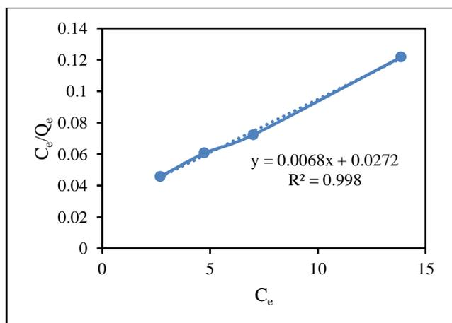
Figure 6. Langmuir isotherm adsorption plot
