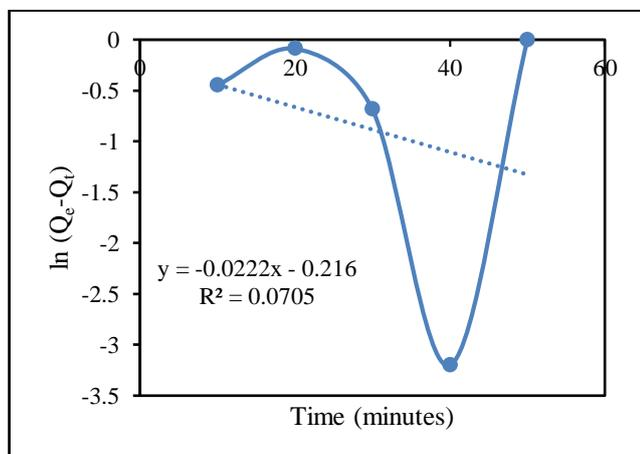
Figure 4. The graph of  $\ln(Q_e - Q_t)$  against time for pseudo-first-order
