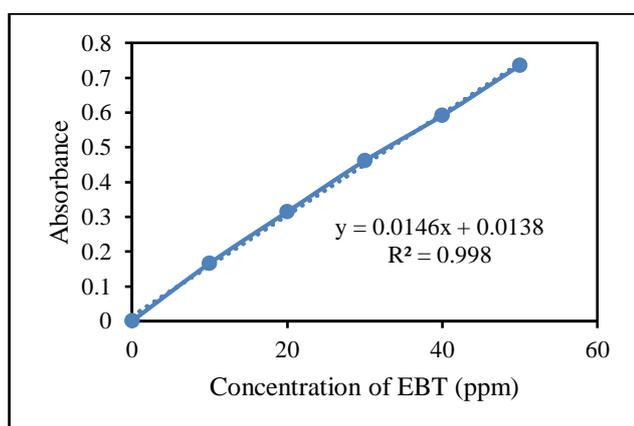
Figure 3. Calibration Curve of EBT standard solutions ( $\lambda_{max} = 541$  nm)
