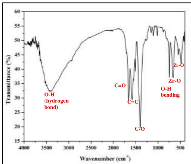
Figure 2. FTIR spectra of Normal UiO-66
