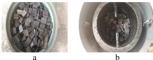
Figure 2. (a). Used tires that have been cut into pieces, (b). Used tires in a pyrolysis reactor
