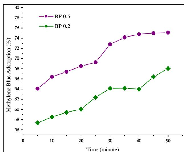
Figure 3. Methylene Blue Adsorption on BP Material
