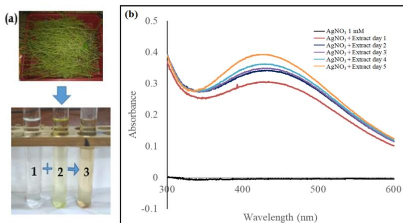
Figure 1. Biosynthesis of silver nanoparticles (a): *Moringa oleifera* leaf stalk waste, aqueous silver nitrate (1), aqueous leaf stalk extract (2), silver nanoparticles (AgNPs) (3); (b): UV-Vis absorbance spectra peak of AgNP at different incubation time.
