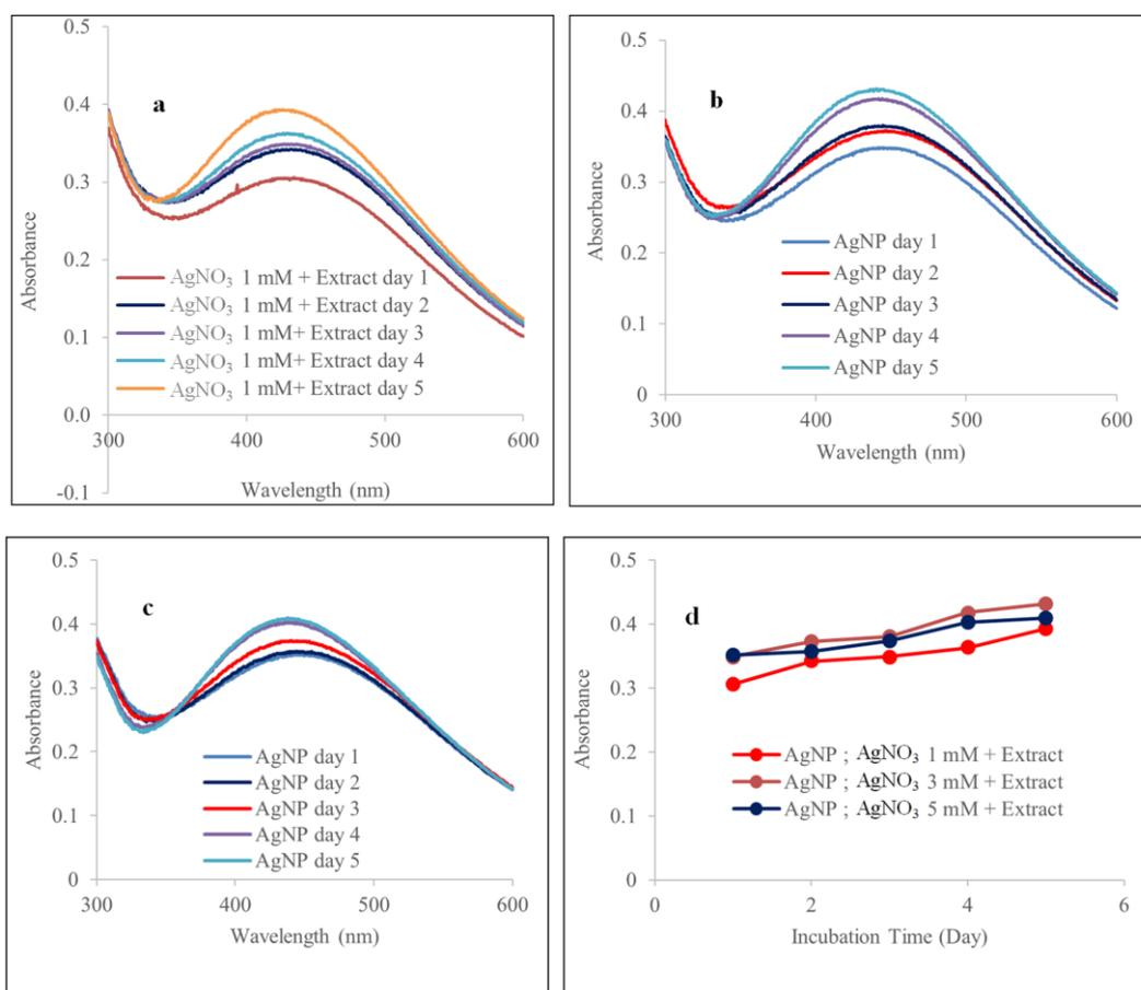
Figure 2. UV-Vis spectra of AgNP during incubation time (a) AgNO<sub>3</sub> 1 mM + *M. oleifera* leaf stalk extract, (b) AgNO<sub>3</sub> 3 mM + *M. oleifera* leaf stalk extract, (c) AgNO<sub>3</sub> 5 mM + *M. oleifera* leaf stalk extract; (d) the change of SPR intensity during reaction time
