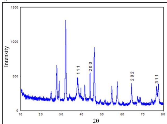
Figure 4. XRD pattern of silver nanoparticle (aqueous  $\text{AgNO}_3$  1 mM + *M. oleifera* leaf stalk aqueous extract)
