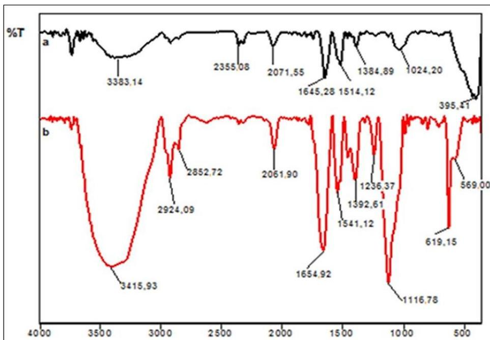
Figure 3. The infrared spectrum (a) silver nanoparticles, (b) Moringa leaf stalk extract
