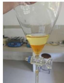
Figure 3. Results of transesterification: top layer (methyl ester) and down layer (glycerol and residues)
