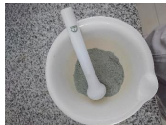
Figure 1. Natural Zeolite Size Reduction
