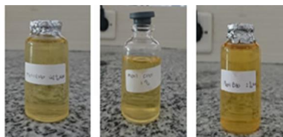
Figure 4. Results of the transesterification reaction after washing and heating (left to right respectively: 0.8; 1.0; and 2% of KOH)
