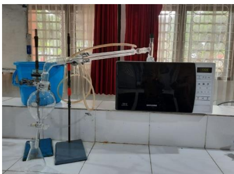
Figure 1. Microwave Assisted Hydrodistillation (MAHD) lime peel essential oil
