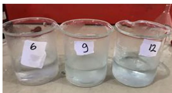
Figure 4. Synthesis of Cu-NPs with variations in pH
