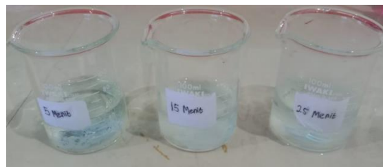
Figure 6. Synthesis of Cu-NPs with variations in stirring time: 5, 15, and 25 minutes
