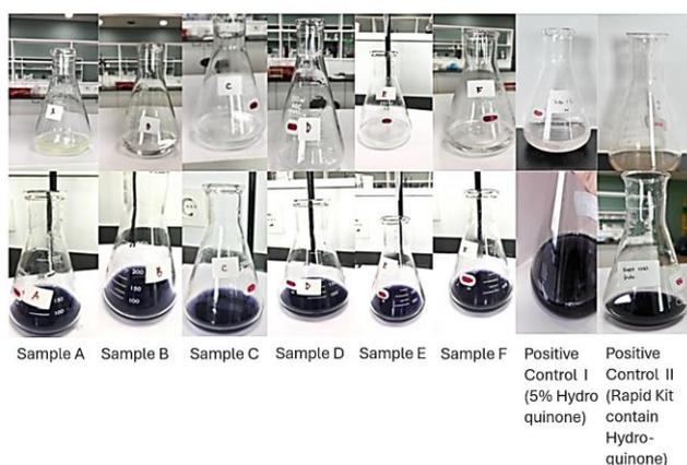
Figure 3. Cerimetry titration result
