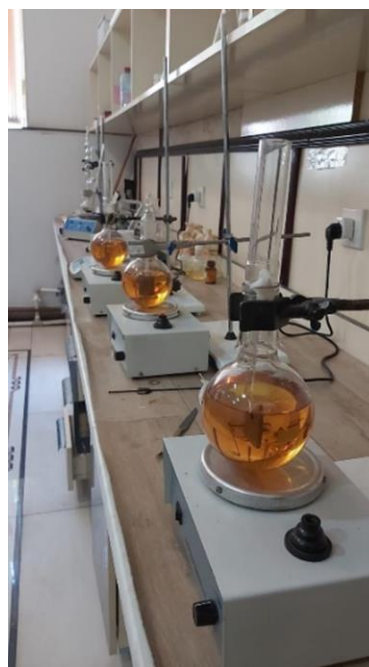
Figure 1. Diesel fuel was tested as a corrosion medium
