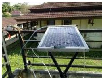
Gambar 1. Panel Surya Dengan *Water Cooling*
