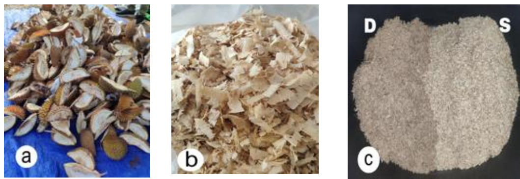
Figure 1. Raw materials and prepared particles: (a) whole durian peel, (b) sengon sawdust, and (c) ground and sieved durian peel (D) and sengon sawdust particles (S)
