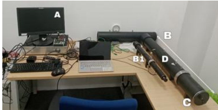
Figure 2. Experimental setup of the two-microphone impedance-tube system: (A) sound source, (B) main impedance tube, (B1) smaller-diameter tube for high-frequency measurements, (C) specimen holder, and (D) microphones.
