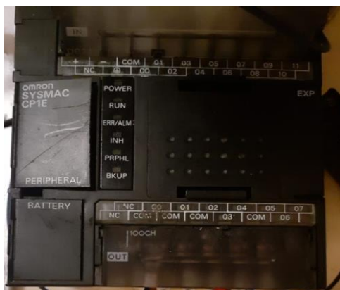
Gambar 5. PLC Omron Sysmac CP1E
