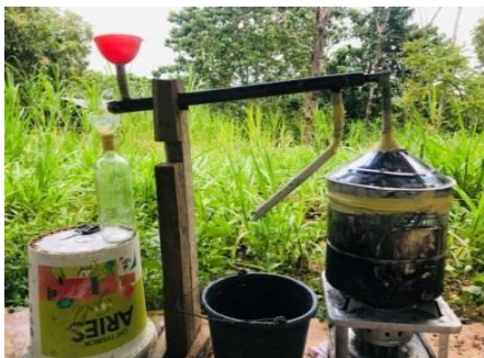
Figure 1. Distillation Equipment Set-up
