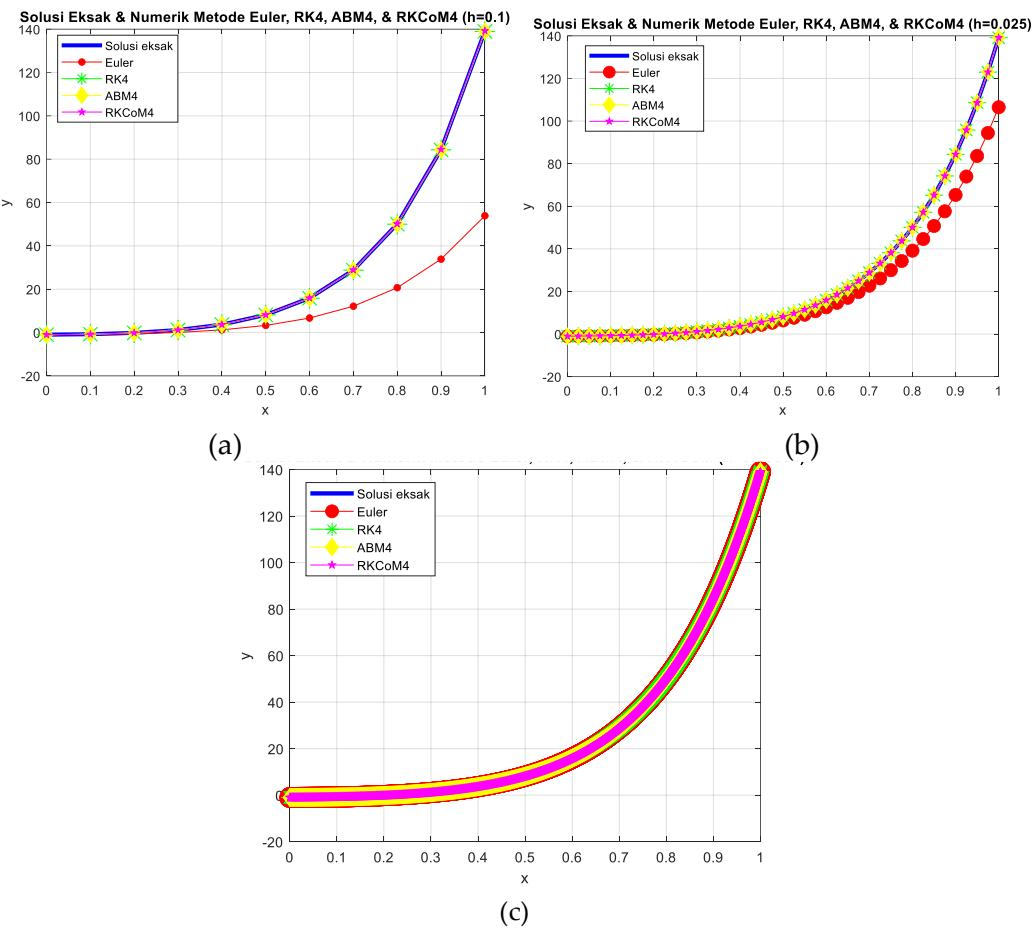
**Figure 1.** Comparison of Exact Solution and Numerical Solution for the case of Equation 1 by Euler, RK4, ABM4, and RKCoM4 methods with different  $h$  values,
